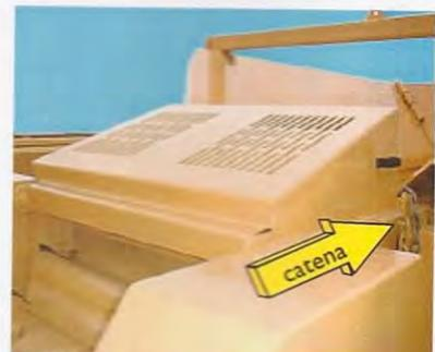
xi) Rotate cover into position & attach chains.
